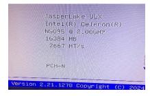
So, there you have it - the machine is a fake 😳 . The machine is, in fact, not based on an Intel i9 8950HK as advertised and/or sold but is based on an Intel Celeron 5095 CPU and GPU. This is a much, much lower grade CPU and GPU.
